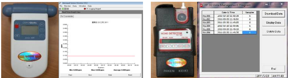
Fig. 11. TVOC Monitor (left)/HCHO Detector (right)
