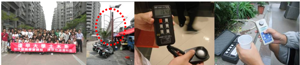
Fig. 16. The author led students to perform noise tests on sound-proof walls, illumination tests in stairways, and turbidity test on public use water
